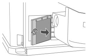
WARNING: DO NOT attempt to remove the assembly until the lamp has fully cooled. If you feel any heat near the lamp, STOP and wait until the lamp has FULLY COOLED.
